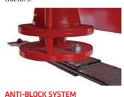
High tensile spindles feature antiwrap pins preventing frustrating blockages around spindles in extreme conditions.
