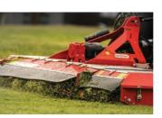
**GREATER MOWING VERSATILITY** The improved cutting chamber and baffle design directs airflow from the blades out and over the rear roller for a better cut and spread.
