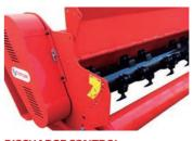
HYDRAULIC SIDE SHIFT The Warlord can be quickly offset to the right by up to 500mm. Perfect for transport and manoeuvring around obstacles whilst mowing.
